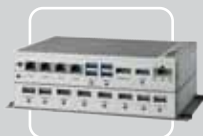
UNO-2484G-6732H5AE · 4 x GbE, 4 x USB 3.0, 4 x USB 2.0, 5x HDMI, 1 x DP (4K), 4 x RS232/422/485
